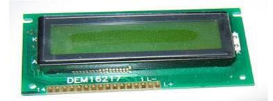
Fig.2(b): Alphanumeric LCD
