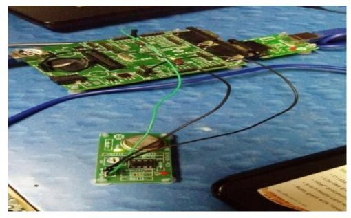
Fig.3: Gas sensor connected to LPC214 microcontroller.
